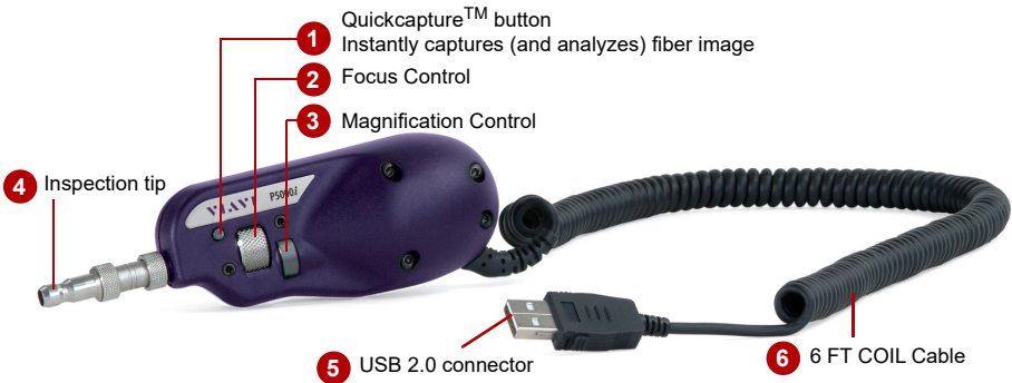
Figure 15 P5000i Probe components
